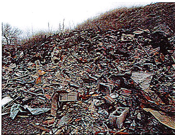
Close-up images of burnt debris: stovetop, brick, wiring, painted wood, and other C&D debris present
