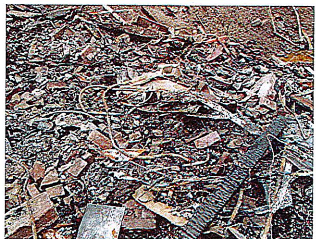
Close-up images of burnt debris: stovetop, brick, wiring, painted wood, and other C&D debris present
